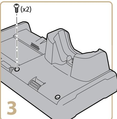
The illustrations show how to install a CN70 computer cup in the DX2 dock. Install all other computer and battery cups the same way.
