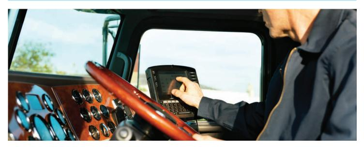
The VC6096 reaches beyond the limited 'silo' of benefits that point solutions offer, allowing businesses to deploy a single device capable of supporting the enterprise applications that are required to collect virtually all available business data from the trucks — from telematics and GPS location-based information to proof of delivery, proof of condition and more.
